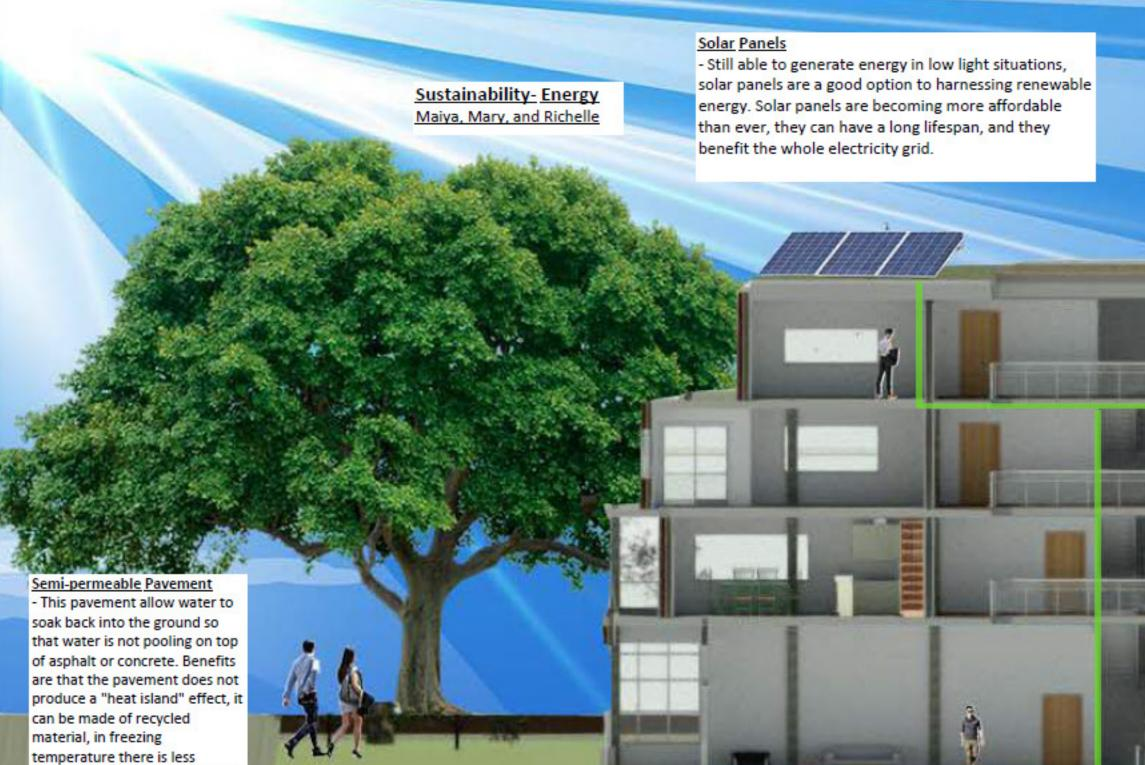
chance that ice will build up on the surface due to porous material and warm ground temperature, and the pavement stays cool in the summers.
